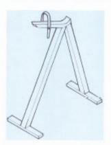
As the shape of the design of bike holder that I have chosen necessitates it to be cast, aluminium will be used for this as it is easier to use due to its lower melting point and often produces a better finish. It is also plenty strong and hard enough for the intended use where the brittleness of cast iron would be a disadvantage. Once the bike holder has been cast, the softer aluminium will also be much easier to work with than the high carbon content steel used.
