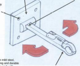
Could be made from mild steel, which would be strong and durable yet relatively easy to work with.
